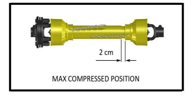
A driveshaft too long may cause structural damages to the tractor and machine. If the driveshaft is too long, it may be adapted by removing it and shortening the tubes according to the instructions provided by the manufacturer in its use and maintenance manual.
